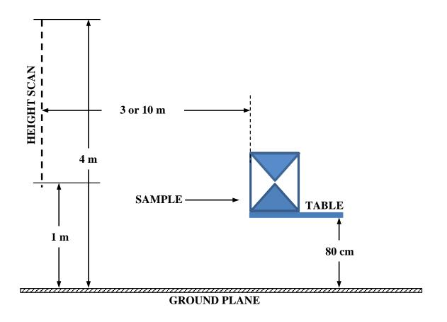
30 to 1000 MHz frequency rage, semi-anechoic room (3 or 10 m)
