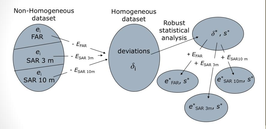
Frequency dependent corrections from FAR to SAR (3 m and 10 m distances and antenna scanning from 1 m to 4 m) are analytically known for short dipoles and applied. This permits to statistically process inhomogeneous data.
